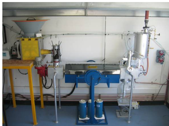
Figure 2: Stage II – small-scale continuous pyrolysis unit
